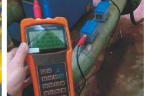
Ultrasonic flow meter for clean water measurement
