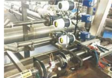
Magnetic flowmeter in calibration
