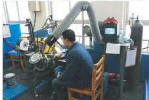
Flowmeter Welding Process
